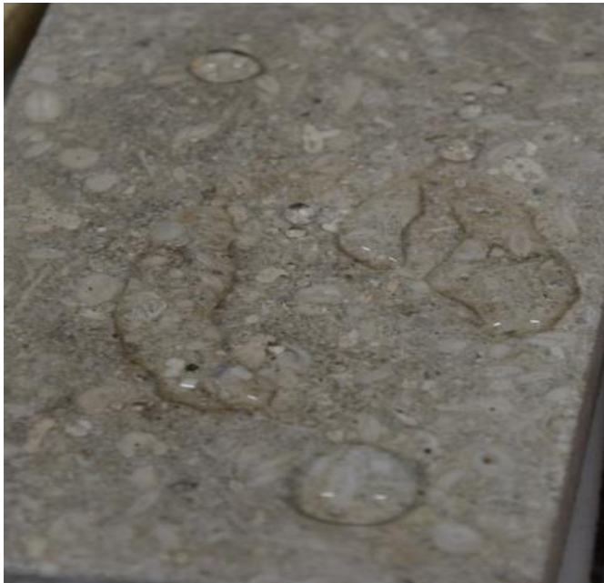
Beading effect on pure limestone and brick (1 days from the treatment)
