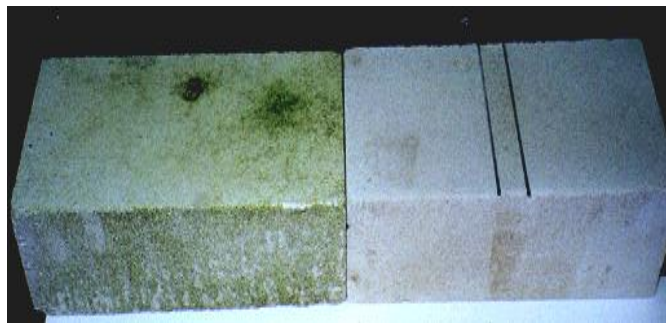
untreated treated Exposure: 3 months under tree
