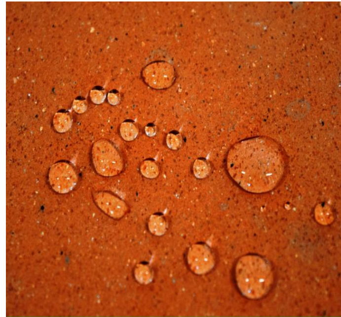
Beading effect on pure limestone and brick (1 days from the treatment)
