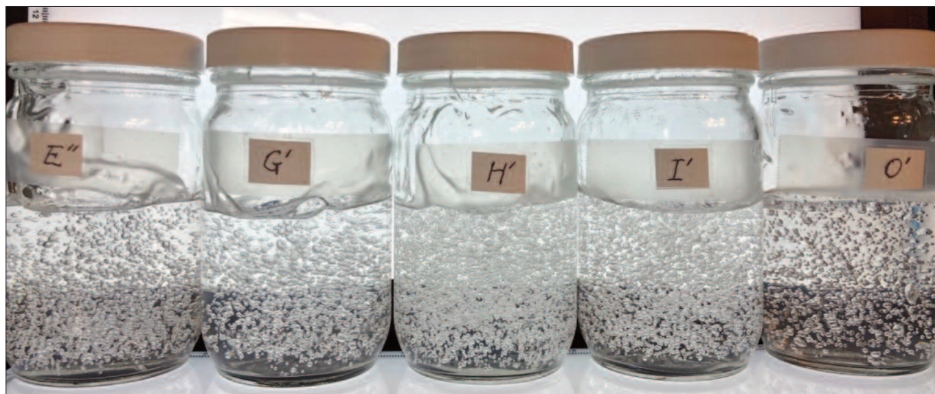
Figure 5: BRB Clear Hand Sanitization Gels containing 2% of: (E') PEG-12 Dimethicone; (G') Blank; (H') PEG-10 Dimethicone; (I') PEG/PPG-18/18 Dimethicone; (O') PG/Glycerin.
